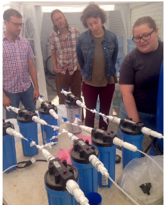
From left: Dr. Polizzotto, Dr. Kerans, and Maia Fitzstevens of NC State University work with Sarah Mitchell of Engineers Without Borders UK on the lead-lag adsorbers at the Caminos de Agua lab.
