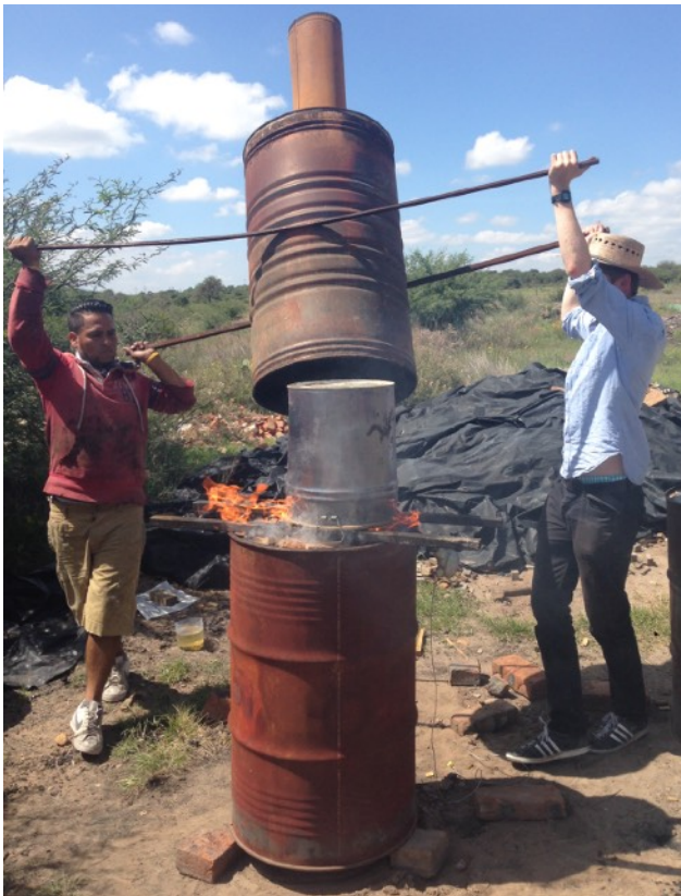
Top left: Caminos staff cover the bone retort with the combustion chamber during a bone char burn; Top right: TLUD-K bone char gasifier ready to be moved over to the second fuel chamber/gasifier.
