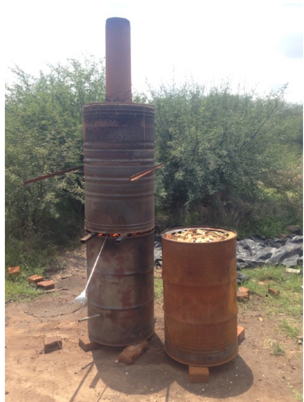
Top left: Caminos staff cover the bone retort with the combustion chamber during a bone char burn; Top right: TLUD-K bone char gasifier ready to be moved over to the second fuel chamber/gasifier.
