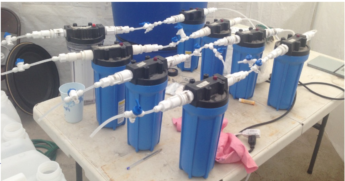
Four prototype column set-up in lead-lag for testing fluoride and arsenic adsorption.
